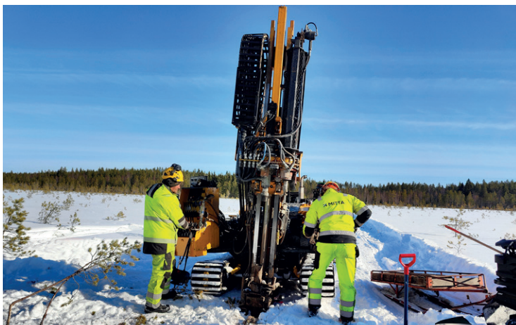
Mitta Oy crew and base-of-till and top-of-rock sampling rig operating at Kiimala Trend's Pääneva prospect during the quarter.
